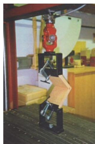
Applied load in compression. Test component - Beech - Glued - dowel joint.
